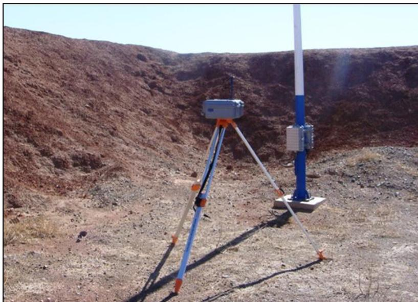
The Dust Trak™ monitoring device is placed at each monitoring location for a 24-hour measurement period. Dust deposition was measured using a dust deposition gauge, as presented in *Figure 3.4*.
